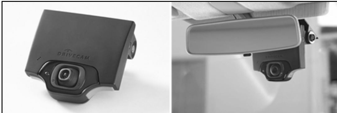
Figure 1. Image. Event Recorder (Left) and Typical Installation of Event Recorder behind the Vehicle's Rearview Mirror (Right)
