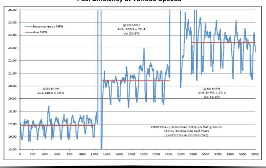
Figure 4 Fuel Efficiency at Various Speeds<sup>xv</sup>
