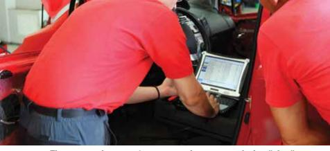
There is a wide array of automotive diagnostic tools that "plug" into a vehicle to speed the process of diagnosing and identifying issues and fault codes.
