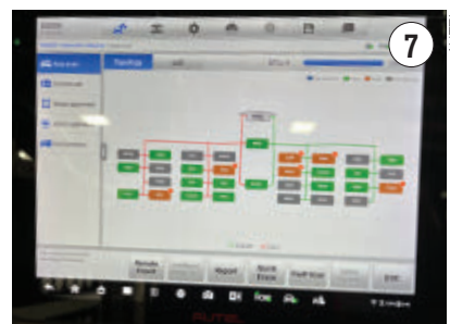
THIS TOPOLOGY MAP demonstrates how many computers communicate together on this vehicle and the complexity of the networks they communicate on.
