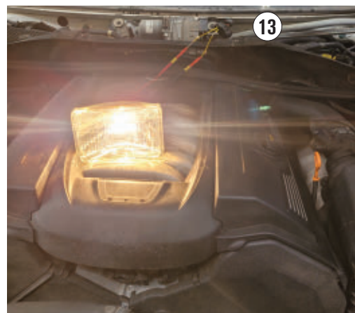
THIS SEALED HEADLAMP bulb provided the electrical load for the wiper motor circuit. Testing in this fashion loads the circuit dynamically and is a more accurate way of determining the health of the entire circuit prior to replacing a failed component.
