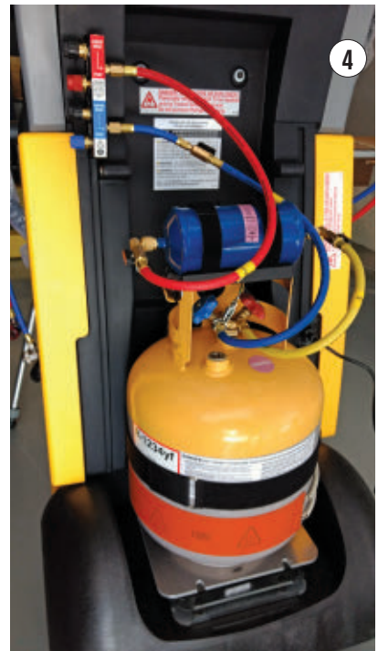
SWITCHING FROM R-134A TO R-1234YF requires changing the rear tank on this CPS FX3030 recovery machine.
