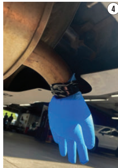
OLD SCHOOL BUT effective! There is a compression leak through the exhaust valve.
