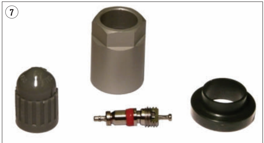
ALWAYS USE A SERVICE KIT when repairing a tire with a metal TPMS valve stem. These parts can become damaged due to corrosion, causing a leak. Rubber TPMS valve stems do not corrode.
