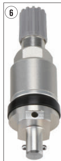
CLAMP-IN SENSORS are subject to galvanic corrosion when exposed to road salt and moisture. Corrosion can weaken the valve stem, leading to a possible sudden loss of tire pressure. Courtesy of Autel.
