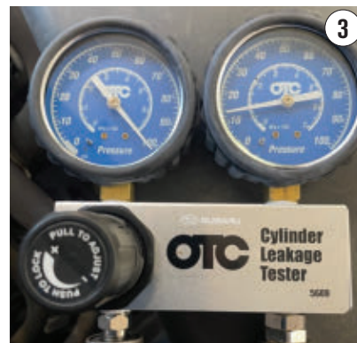
CYLINDER LEAKAGE results for cylinder one.
