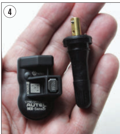
THIS MX 1-SENSOR by Autel has both 315MHz and 433 MHz frequencies; is 100% ID cloneable with no relearn required, and can be programmed and updated with Autel wireless programming tools. The PRESS release valve stem allows rubber and metal valve stems to be interchanged by hand.
