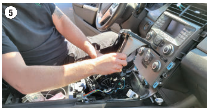
A DEFECTIVE SWITCH was the root cause of the parasitic drain.
