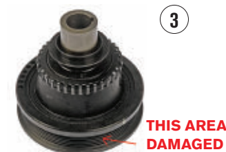
THE AREA INDICATED BY THE RED ARROW was damaged, and the harmonic balancer required replacement.
