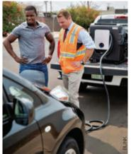
AS EVS BECOME MORE COM-MON, more drivers will miscalculate the range of their cars and get stuck with no charge. Blink offers a portable emergency charger that supports 240V AC charging providing up to 9.6kW of charge (about one mile per minute of charging). The unit has a gasoline engine that powers a generator.
