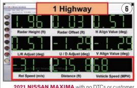
**2021 NISSAN MAXIMA** with no DTCs or customer complaints, using Adaptive Cruise Control, first (above) and second (below) captures.
