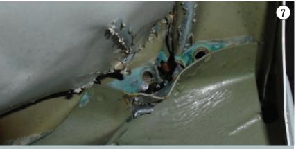
**DAMAGE UNDER THE RIGHT REAR** of a Lincoln SUV causing the liftgate to be out of alignment.
