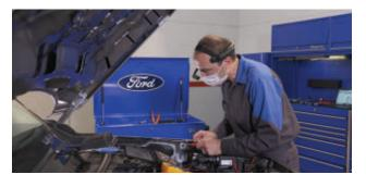
on the vehicle in real time. SWIS's augmented reality capability allows TAC team members to display modified or enhanced images on the headset for the dealer technicians to view.
