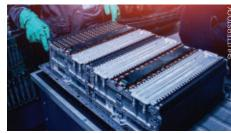
**AN EV TECHNICIAN SERVICING** a high voltage battery.
