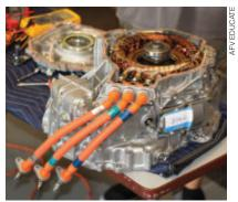
**AN ELECTRIC MOTOR** from a Toyota Prius. The Prius has two electric motor/generators and a gasoline engine.
