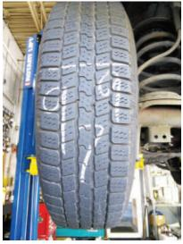
MEASURE TIRES ACROSS THE TREAD and write the measurement in 32nds in chalk on the tread. Each subsequent inspection will show the number(s) going down, counting down till "retirement."
