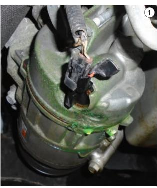
LEAKAGE FROM A PTU that caused a burning smell from the exhaust system after the technician repaired a burning smell from the brakes.
