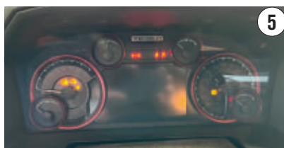
THE INSTRUMENT CLUSTER completely shut down due to the network crashing.
