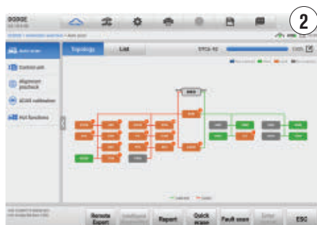
THIS IS THE FIRST FULL VEHICLE SCAN that we did on the vehicle after the customer reported the problem. I did not include all the codes, as there are too many to show in one picture.
