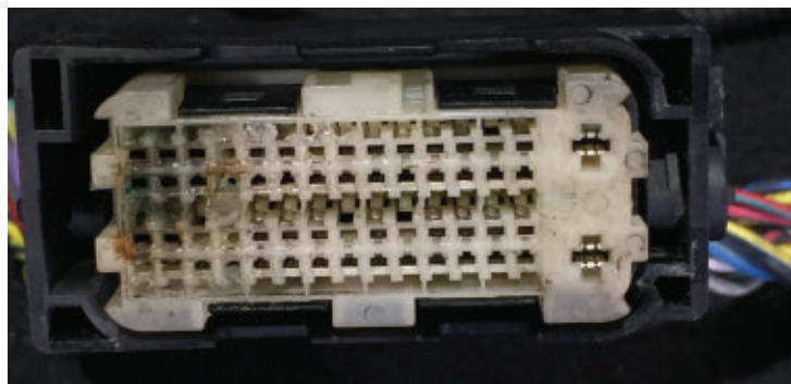
A CONNECTOR to the engine control unit that has damage to the terminals.
