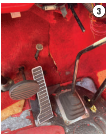
THIS IS LIKELY THE OLDEST versions of push-to-start, seen here above the accelerator pedal.
