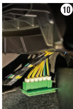
THIS IS A PICTURE of the passenger side CAN bus Star connector. It is located against the right front of a pillar. You can see the edge of the blower motor off to the one side.
