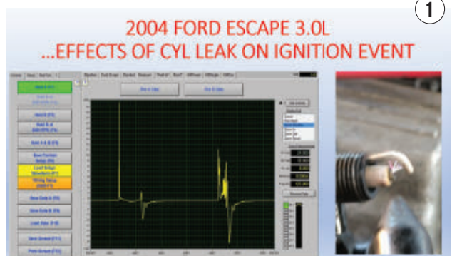
THE IGNITION EVENT is being captured on a DSO simultaneously as shop air is blown across a firing spark plug. This simulates what occurs in the cylinder during a compression leak.
