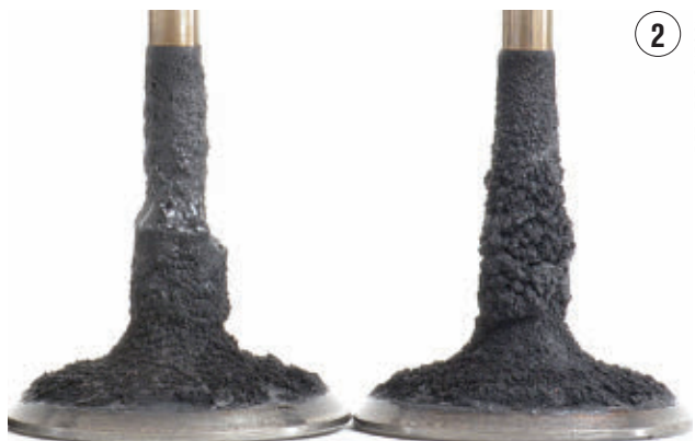
VALVE CARBON DEPOSITS in GDI engines can cause the air to tumble into the combustion chamber and disrupt the combustion process, which generates misfires.
