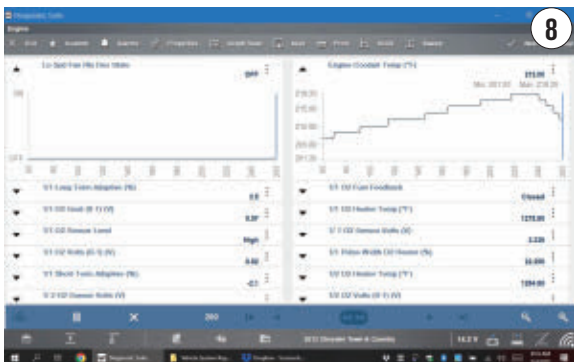
THE PIDS DISPLAYING ADEQUATE TEMPERATURE to operate the fans, but no command being give. This offers insight to a computer related fault.
