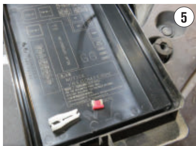
5 INSPECTING THE UNDER-HOOD FUSE BLOCK confirmed my suspicion was correct. The 10A Ignition supply fuse used by all six coils was now open due to excessive amperage.
