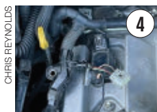
4 WHILE LOCATING AN EASY POINT of access for measurable coil readings, I found a non-OEM modification to two wires on Ignition Coil 1. These two wires were for coil power supply and coil round supply.
