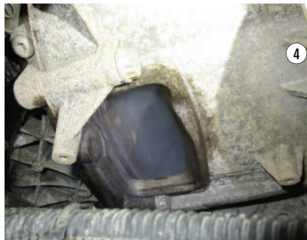
THE PRESENCE OF SMOKE in the bell housing is indicative of a rear main crankshaft seal leak, as smoke is being introduced to the crankcase/PCV system.
