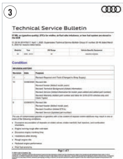
THIS TSB INDICATES a potential cause for driveability faults may be linked to gasoline quality and/or induction system carbon build-up.
