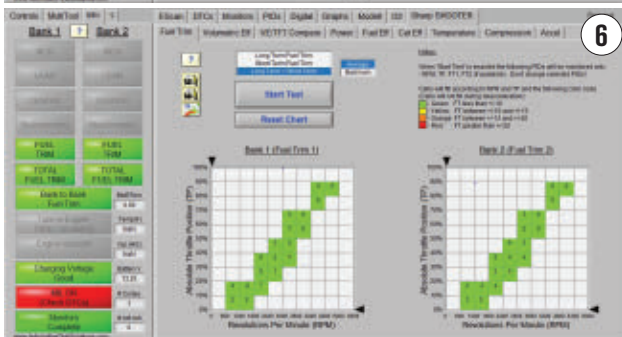
PROPER FUEL TRIM DISPLAYED HERE indicates the fuel being delivered to the cylinders is correct for the operating conditions, throughout the entire rpm/load range.
