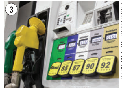
WHILE IT WOULD BE DIFFICULT to get the larger diesel fuel pump nozzle to fit into a gasoline vehicle's smaller diameter filler neck, the opposite (gas accidentally pumped into a diesel fuel tank), E85 would be easy to pump into a non-flex fuel vehicle. Either way, a complete fuel system flush would need to be performed in addition to repairing the damage the wrong fuel might cause.
