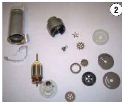
AFTER THE ELECTRIC PUMP is removed from the plastic module assembly, the metal cylindrical electric pump can be snipped (as shown) or scored with a pipe cutter (heavier cast body motors) to be completely dissected to inspect the impeller, turbine, check valve and armature/brushes.
