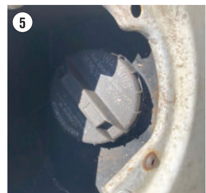
FUEL TANK FILLER NECK OPENINGS are another possible path for environmental contamination.
