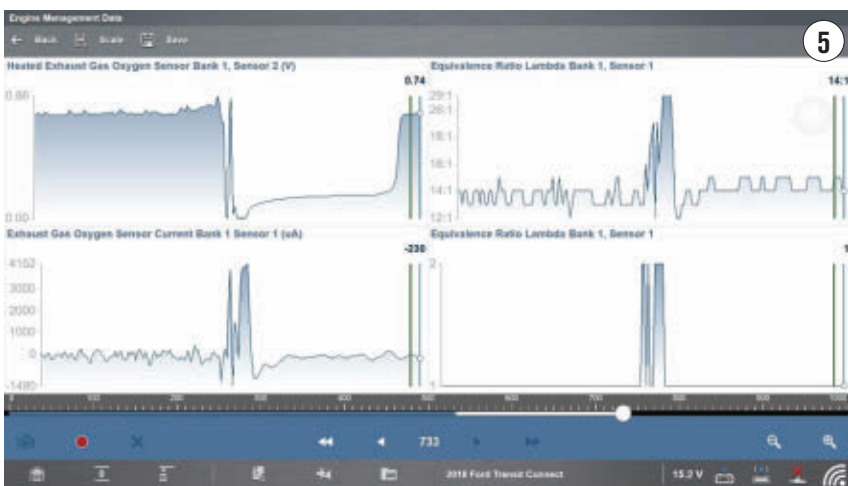
THIS SCREENSHOT DEMONSTRATES a manual oxygen storage capacity test result for a catalytic converter.
