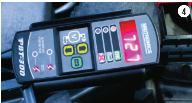
FIGURE 4- THE MIDTRONICS PBT-300 computerized battery, starting, and charging system tool.
