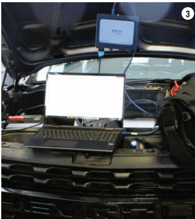
THE BEGINNING OF LAB SCOPE SET UP. The starter circuit and components can easily be evaluated right from under the hood with minimal effort or time invested.
