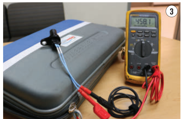
USING A DMM TO MEASURE STATIC RESISTANCE can provide a critical clue when diagnosing sensor low or no output concerns. This sensor displays a resistive value well within the normalized range of 200-1,000 ohms.
