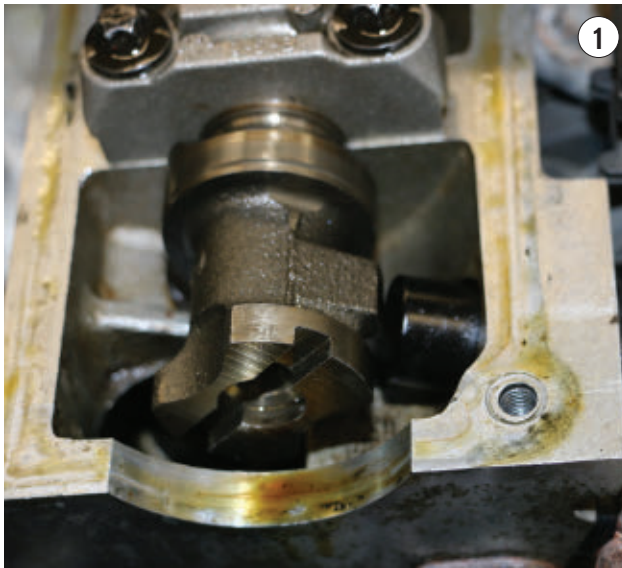
THIS TWO-WIRE , variable reluctance sensor generates an analog voltage output to locate the intake camshaft position on a 2.0L Ford Zetec engine.
