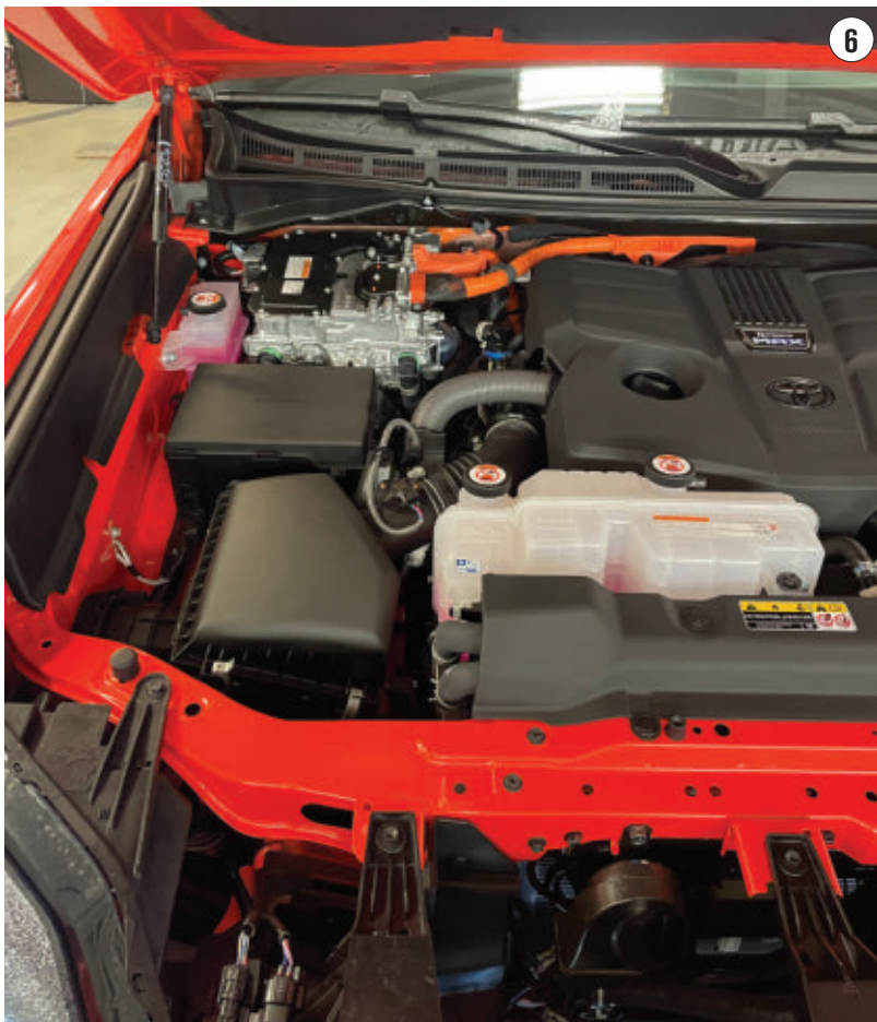
HYBRID INVERTER LOCATED on the passenger side of the engine compartment along the firewall.
