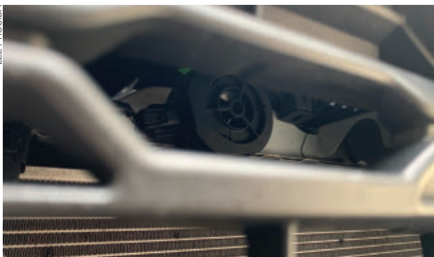
AVAS SPEAKER , as seen through the grille of a Toyota RAV4 Hybrid. On an EV there obviously wouldn't be a grille, so the speakers are often mounted behind body paneling or beneath the vehicle.
