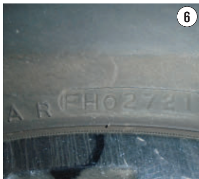
BUILD DATE STAMPED on the sidewall of a tire. This tire was manufactured during the 27th week of 2021.
