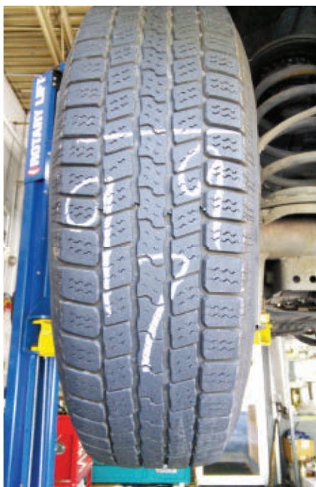
MEASURE TIRES ACROSS THE TREAD and write the measurement in 32nds in chalk on the tread. Each subsequent inspection will show the number(s) going down, counting down till "retirement".
