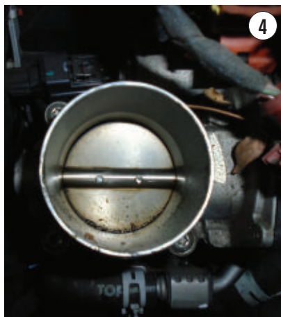
THROTTLE BODY SLUDGE blocks idle air and possibly changes the TPS value at idle.
