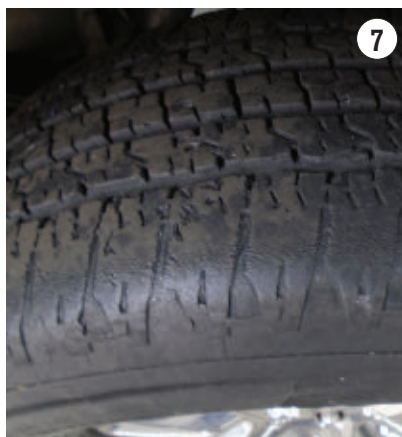
THIS ROTTING AND CRACKING is why you should look past the tire tread and scrutinize the entire tire.
