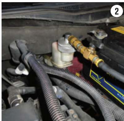
BRAKE PRESSURE BLEEDER hooked up to a master cylinder reservoir. A pressure bleeder is the best way to replace the brake fluid.
