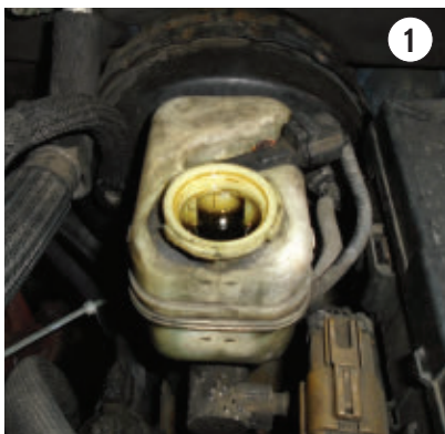
BRAKE FLUID that has absorbed water becomes dark and murky. It should be changed before it damages hydraulic brake components.
