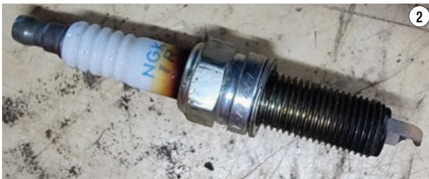
COMBUSTION GASES are passing through the spark plug and leaving soot-like evidence behind on the insulator.
