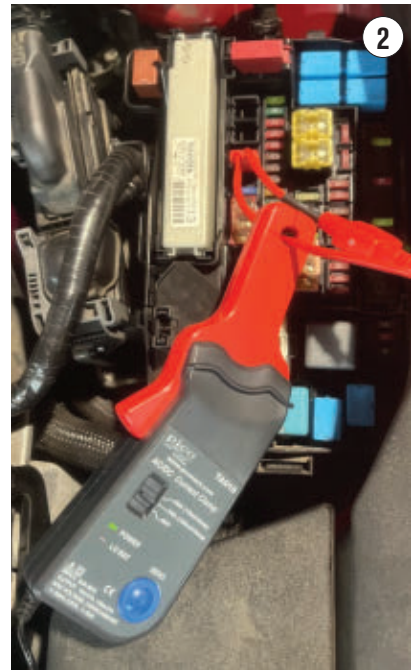
THE AMP PROBE DEMONSTRATES the work being performed in the circuit being measured. Since the current flow is the same anywhere in the series circuit, this measurement can be acquired at the most convenient location to save time and energy.
