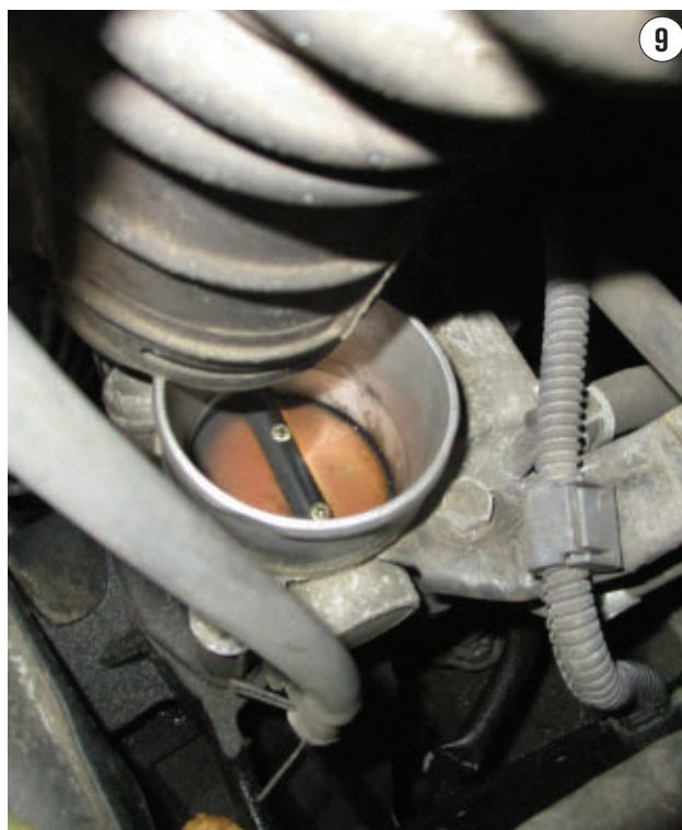
THIS COKED-UP THROTTLE VALVE prevented the engine from idling properly and was the root cause of the charging system fault.
