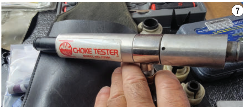
THIS OLD CHOKE TESTER (FOR CARBURETOR TUNING) was used to chill /heat the suspect MAP sensor, proving the fault was temperature related.
