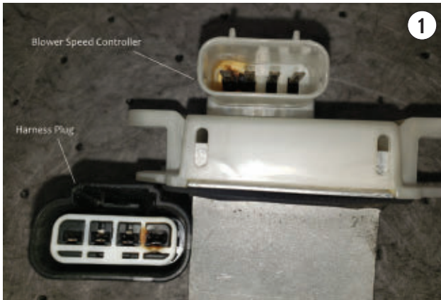
THIS BLOWER SPEED CONTROLLER and harness connector melted from excessive heat caused by resistance in the controller.
