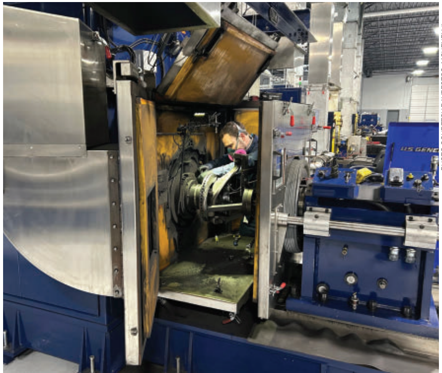
A TECHNICIAN TESTS BRAKE PADS with this Link Engineering brake dynamometer that simulates driving conditions and assesses stopping ability, noise, durability and heat ranges of brake pads.
