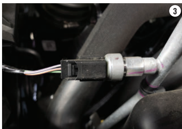
AIR CONDITIONING PRESSURE TRANSDUCER located on the discharge line between the compressor and the condenser.
