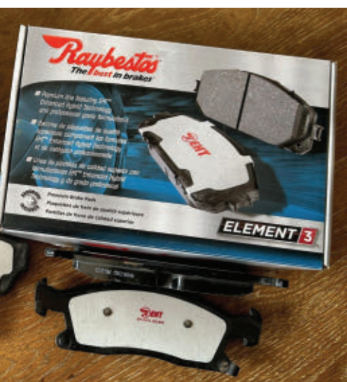
RAYBESTOS ELEMENT3 BRAKE PADS use a hybrid combination of semi-metallic and ceramic compounds in their friction material.
