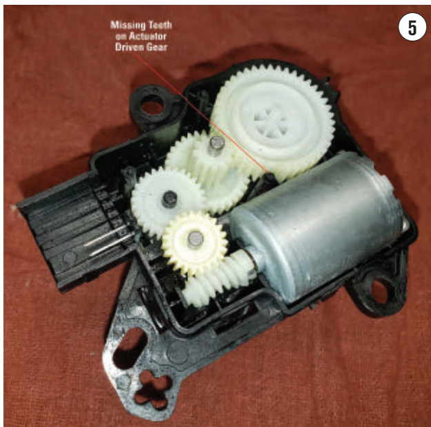
THIS INTERNAL VIEW of an inlet door actuator shows missing teeth on the driven gear, causing the actuator to make a banging noise during operation.
