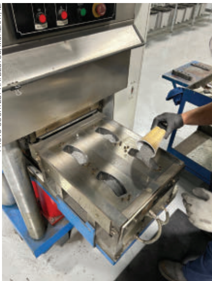
THIS MACHINE IS A POSITIVE MOLD TOOL AND FRICTION HOT PRESS. The pad material mix is poured into the mold cavity and cured using heat and pressure. A set of brake pads can be pressed and cured (heated) in about five minutes.
