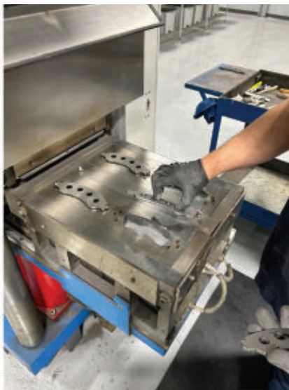
THIS MACHINE IS A POSITIVE MOLD TOOL AND FRICTION HOT PRESS. The pad material mix is poured into the mold cavity and cured using heat and pressure. A set of brake pads can be pressed and cured (heated) in about five minutes.
