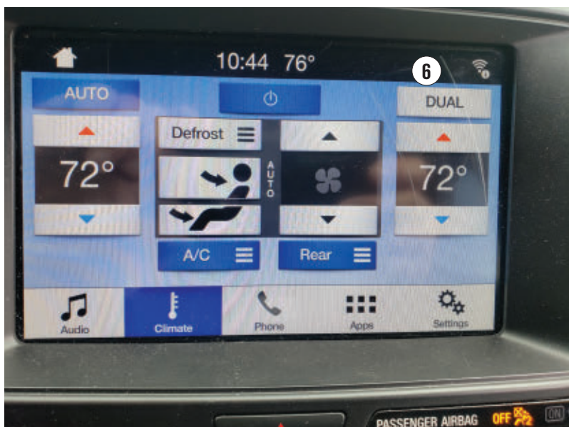
HERE IS THE 8" TOUCHSCREEN opened to the climate control screen on a DATC system.
