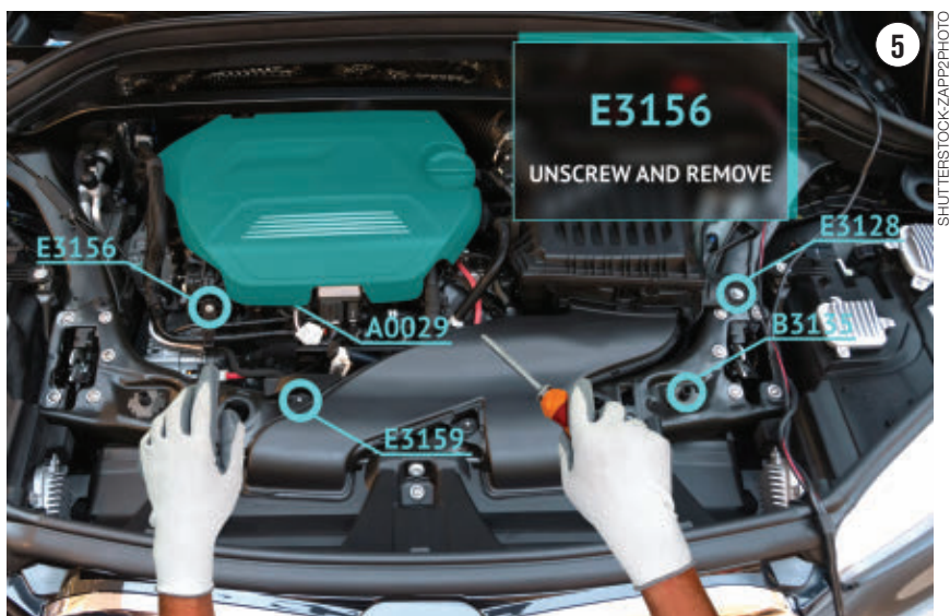
AUGMENTED REALITY being used as an overlay to a client's vehicle for diagnostics.
