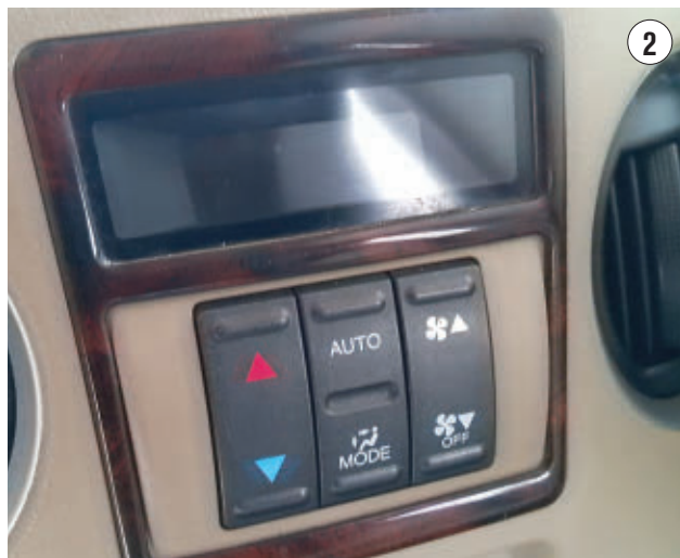
VIEW OF THE REAR CLIMATE CONTROL PANEL during the initial fault (Display is totally blank).
