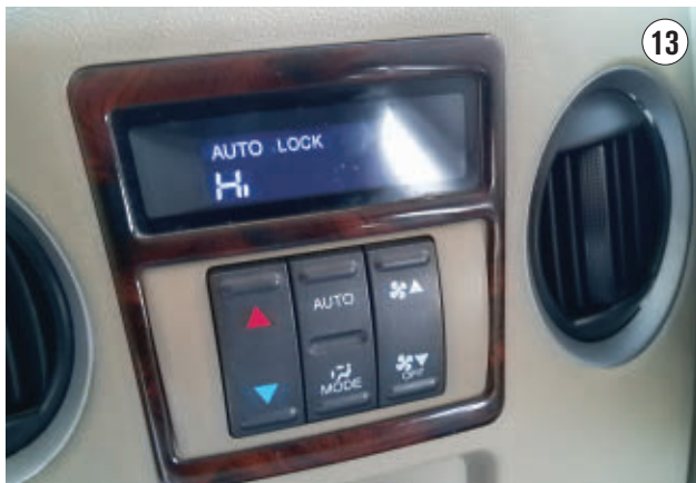
VIEW OF REAR CLIMATE CONTROL with 5V reference restored (display is active).
