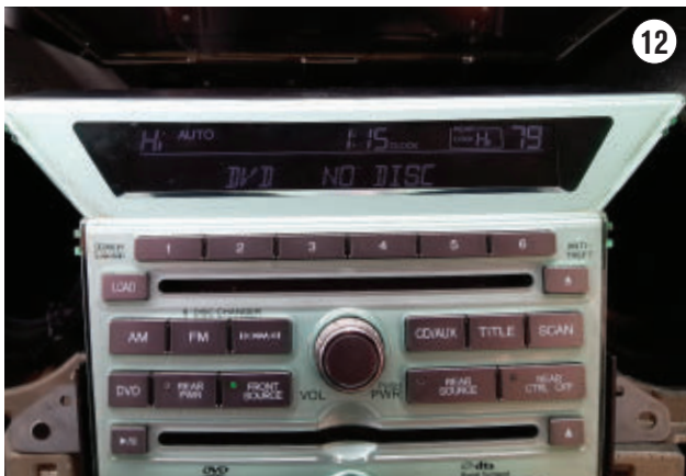
VIEW OF FRONT HVAC MODULE and controls with 5V reference restored (temp displays are now active for driver and passenger front).
