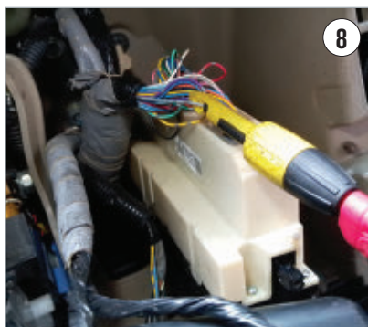
CHANNEL 1 OF MY SCOPE connected to the gray 5V reference wire at the HVAC control unit.
