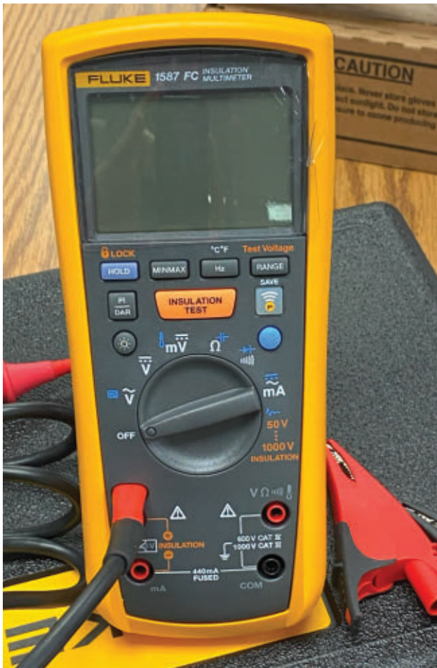
THIS MEGOHMMETER is an insulation tester, an essential tool for determining if a high-voltage component has an unwanted path to chassis ground.
