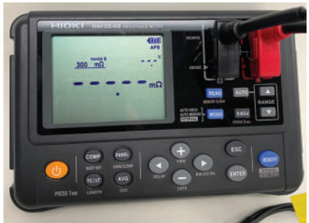
THIS MILLIOHMMETER makes accurate minute measurements of resistance by utilizing a 4-wire test.
