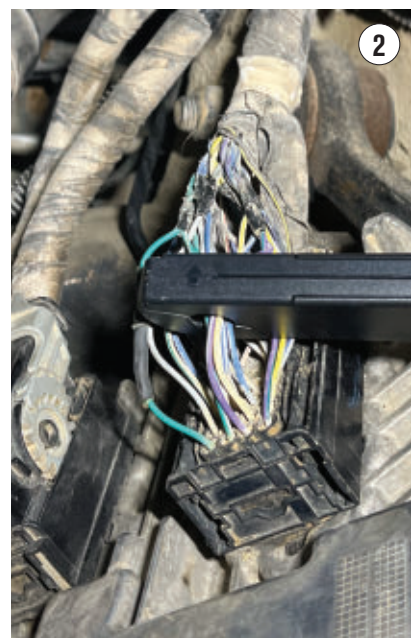
THE INJECTORS' CURRENT FLOW is easily monitored by acquiring the data with a current probe at the ECU.
