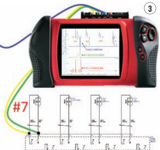
THE INJECTORS' CURRENT FLOW is easily monitored by acquiring the data with a current probe at the ECU.
