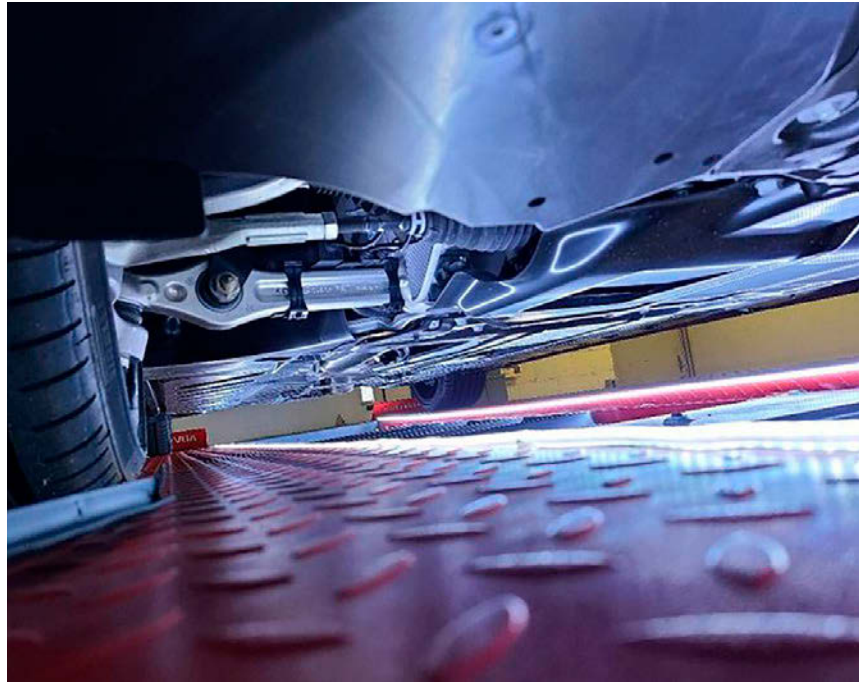
This image shows how brightly lit the underside of a vehicle is when using a lift with LED lights.
