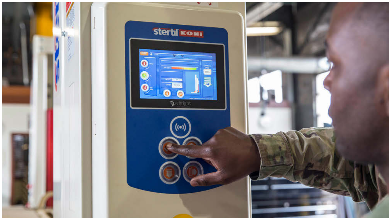
Stertil-Koni's ebright Smart Control System puts all the necessary information on the lifting system at the technician's fingertips.
