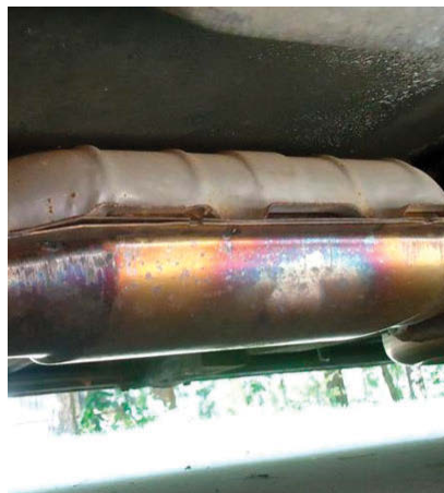
Even slight variations in the air/fuel mixture will cause the converter temperature to rise significantly.
