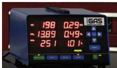
Low HC and CO levels with high NOx emissions are typically not caused by a defective converter.
