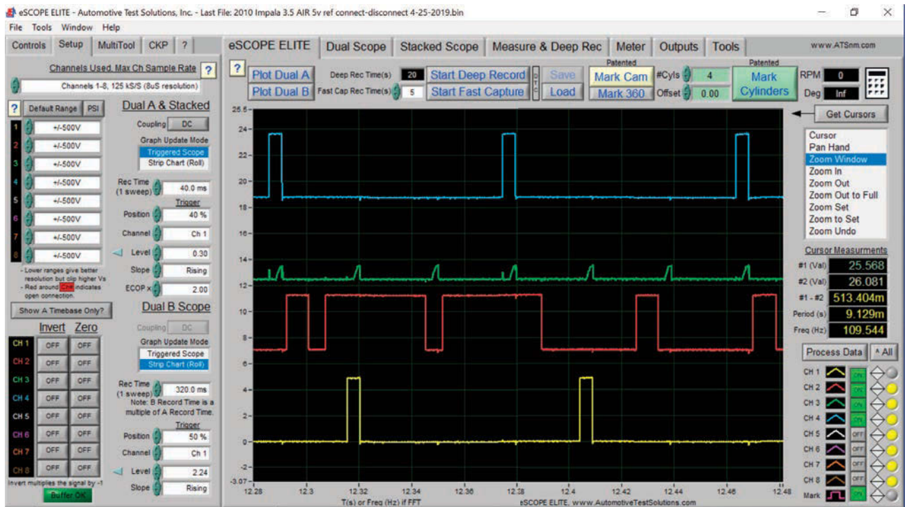
The DSO offers a visual representation of electricity and action/reaction comparative measure of different circuits simultaneously.
