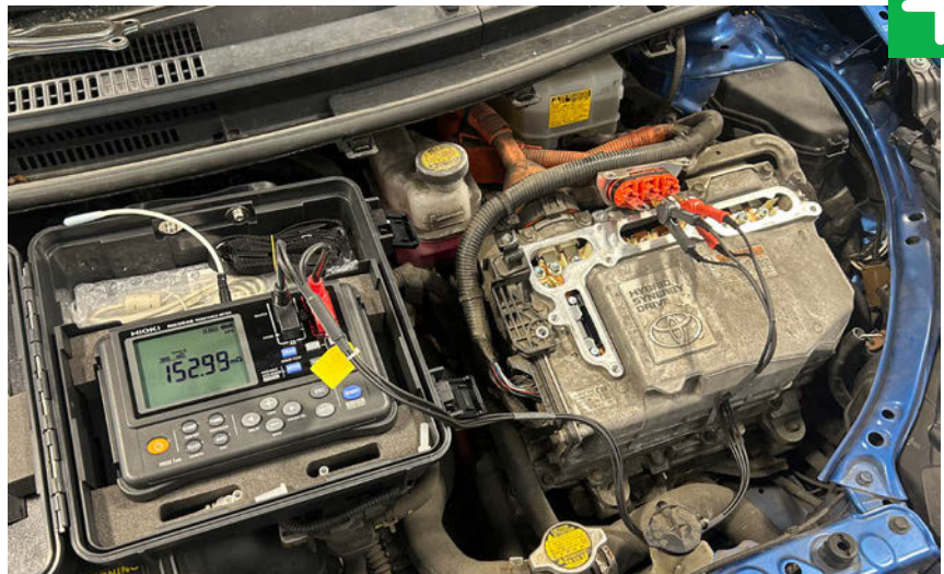
Hioki 3548 showing 152.99 milliohms of U-to-V phase resistances on a 2013 Toyota Prius C. Photo courtesy of Jack Rosebro
