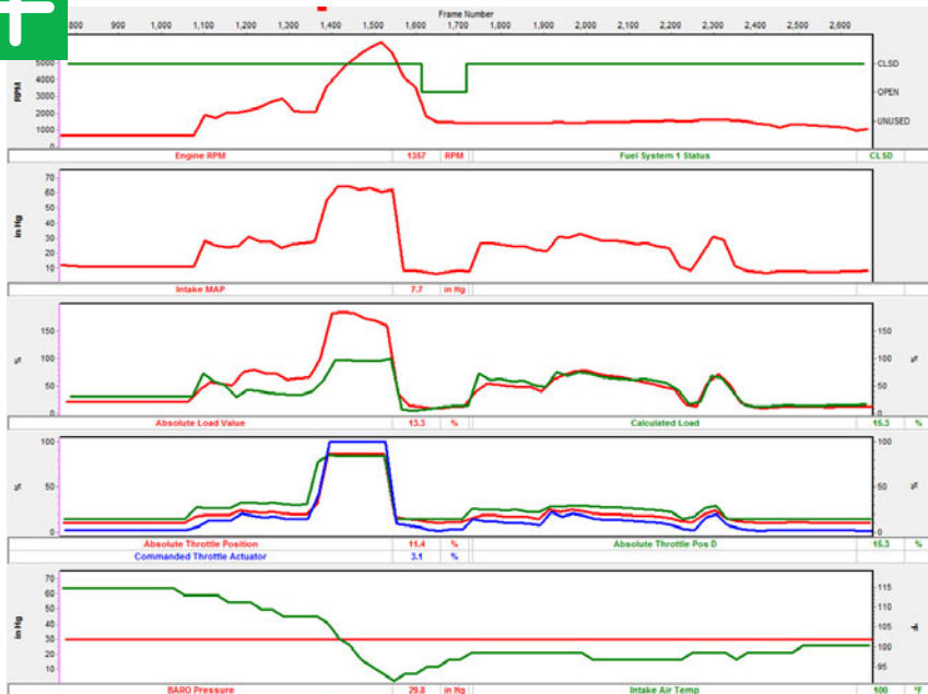
Figure 4— Superimposing line graphs allow an easy-to-compare view of data (like throttle position PIDs) that represents desired and actual positions. If the lines deviate from one another, an underlying fault exists. Photo courtesy of Brandon Steckler
