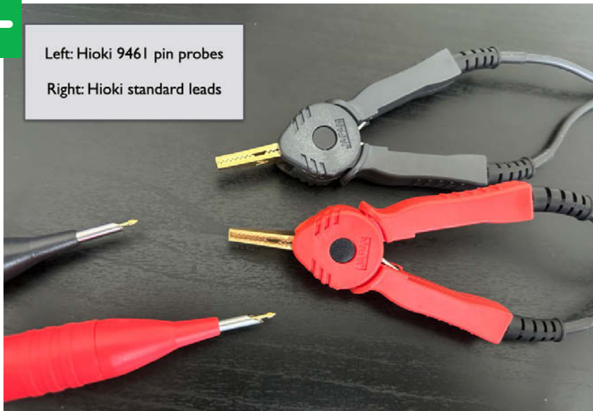
Alligator clip leads are used when measuring phase-to-phase motor-generator resistances. Pin probes are used to measure the resistance of bolted connections, including ground points.
