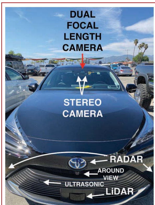
Figure 4 - 2022 Toyota Mirai – ADAS sensor suite including a stereo camera
