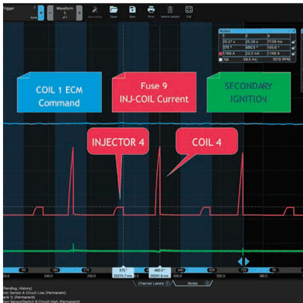
Figure 8 — 2012 Cruze misfire analysis zoom Photo courtesy of Scott Brown
