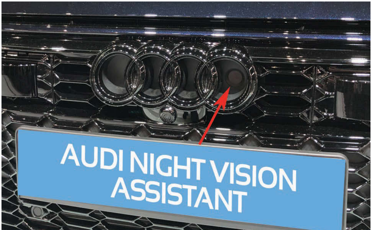
Figure 1 — Audi Night Vision Assistant on a 2019 A6 Photo courtesy of Scott Brown
