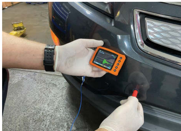
Figure 5 — Ultrasonic sensor testing with AESwave uScope Photo courtesy of Scott Brown
