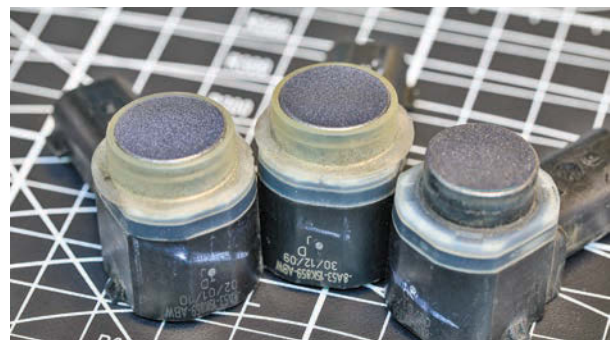
Figure 3 — Ultrasonic sensors - Ford Photo courtesy of Scott Brown
