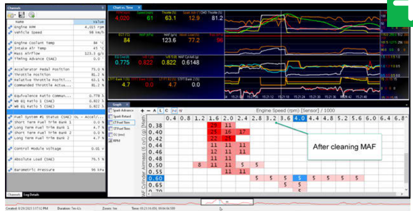
Figure 9 — 2006 Tacoma after MAF sensor cleaning Photo courtesy of Scott Brown
