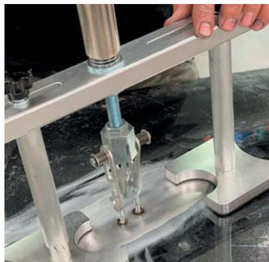
*With the mixed-metal bodies of vehicles nowadays, it's important to have tools that work with different metals such as H&S Autoshot's Aluminum Dent Puller.*
