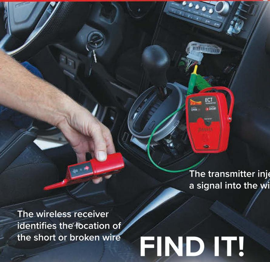
The wireless receiver identifies the location of the short or broken wire
