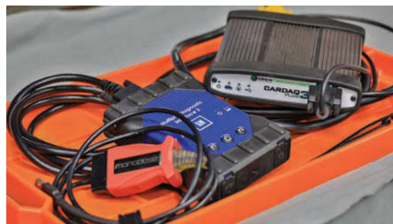
Figure 3- The three programming interfaces: L-R Mongoose Nissan, GM MDI2, and CarDAQ Plus 3
