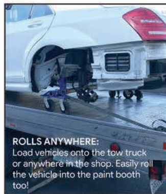
BECOMES PART OF THE VEHICLE: No need to employ any unstable or dangerous lift points. Mounts to the sub frame or cradle using the original mount points and hardware.
