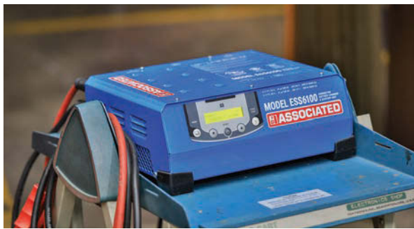
Figure 4 - Programming battery support - Associated Equipment ESS6100
