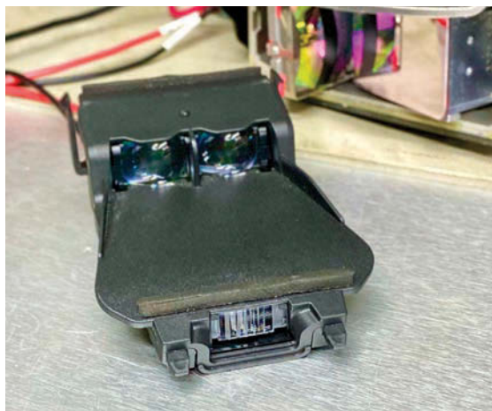
Figure 5- Mazda short range LiDAR sensor; Smart City Brake support
