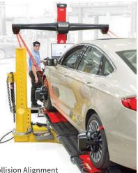
WinAlign17 software. Collision Alignment automatically guides the technician through a workflow of five essential diagnostic measurements, blueprinting the full alignment before work begins. The five measurements are toe out on turn, maximum steer, ride height, suspension body dimension audit, and steering axis inclination.
