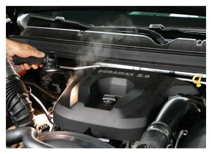
Technicians testing an intake manifold leak using a smoke machine. Photo courtesy of Redline Detection
