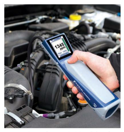
The AST300PPM from INFICON can detect both R-1234yf and R-134a refrigerants. Photo courtesy of INFICON
