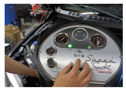
Redline Detection's SpeedSmoke features an onboard air compressor and can handle both low and high pressure testing. Photo courtesy of Redline Detection
