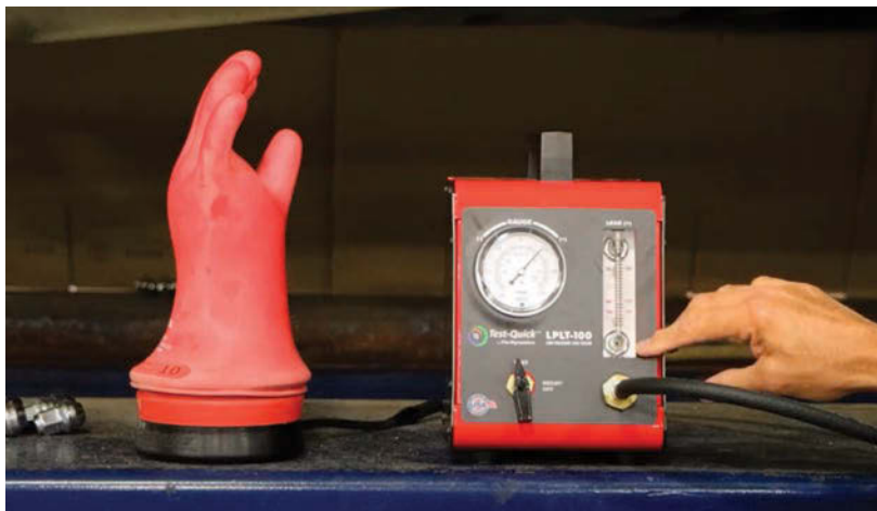
The Flo-Dynamics EV Battery Pack Leak Tester includes a high-voltage glove adapter for technicians to test their gloves. Photo courtesy of Flo-Dynamics
