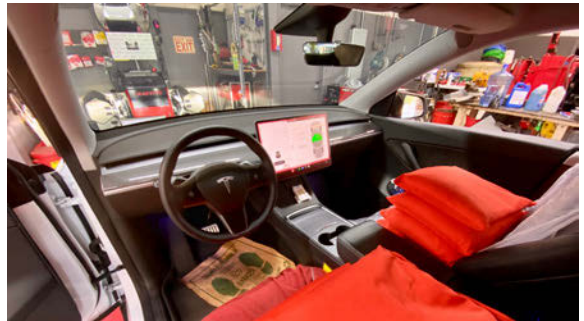
▲ Figure 3 - Properly prepping a Tesla for wheel alignment
