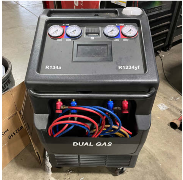
▲ Figure 3 - Ecotecnics Dual Gas A/C machine
