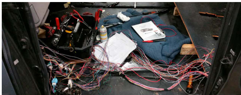
▲ The rear floor was removed to inspect the mating of the original and conversion-harness.
