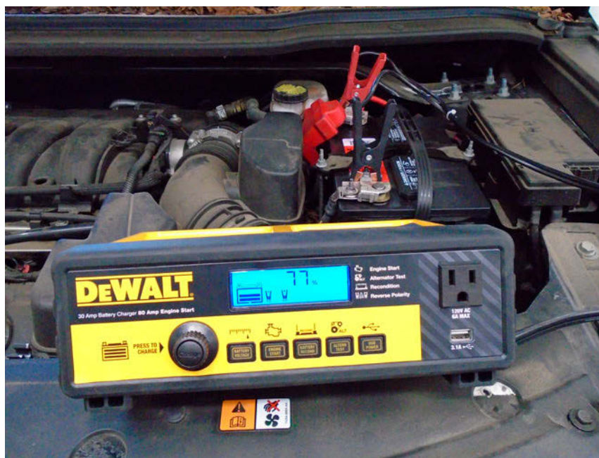
▲ An easy-to-carry battery charger is a great tool to have. This battery is at a 77 percent state of charge, suitable for diagnosing a current draw.
