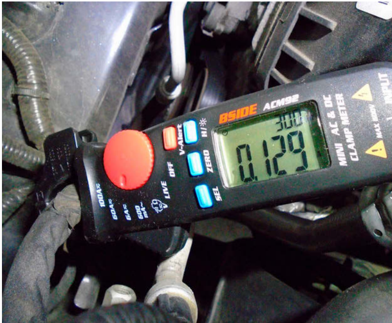
▲ Figure 3 - We had a 129 mA current draw narrowed down to two harnesses. We found the right one using the inductive ammeter.
