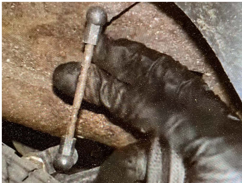
▲ Figure 2— Ride height sensors may be adjustable for rod length. When replacing, measure the original as a reference. If original sensors are removed and reinstalled, be careful to avoid altering rod length.
