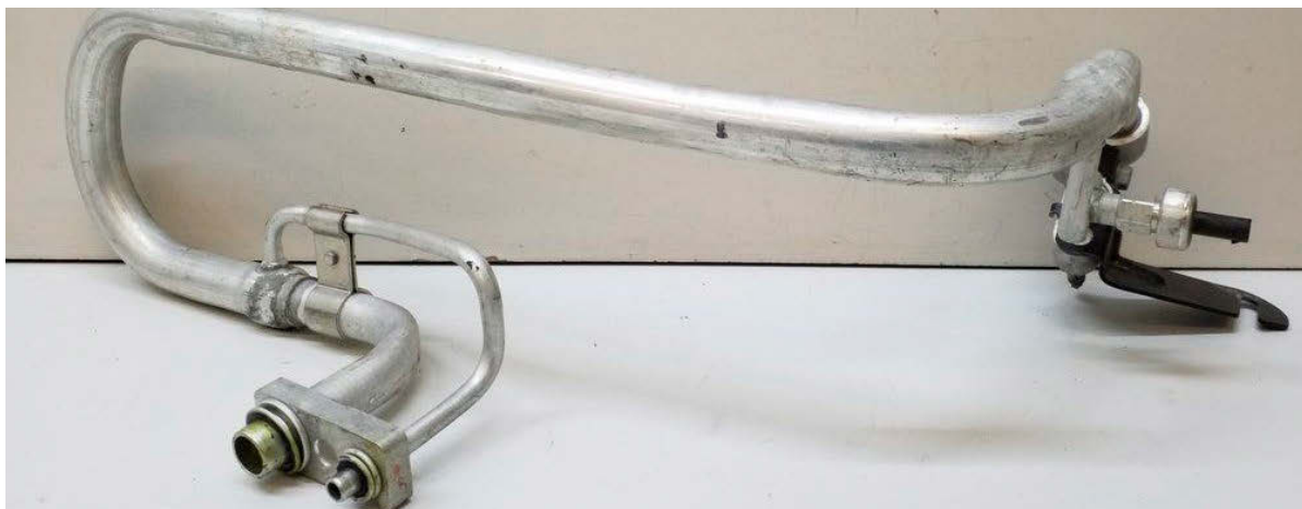
▲ Figure 1 - Chrysler IHX. Note how the design combines the liquid and suction (vapor) lines.
