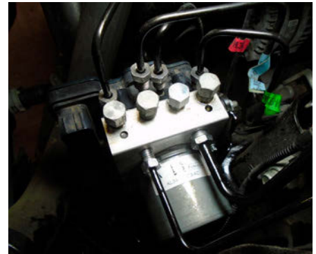
▲ Figure 2 - Image of blockers being used to diagnose an HCU.
