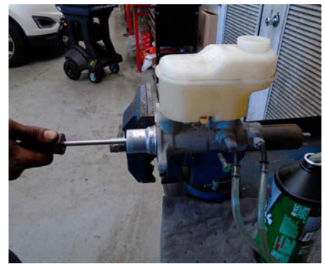
▲ Figure 3 - Bleeding a master cylinder using a bleeding kit with one-way check valves.
