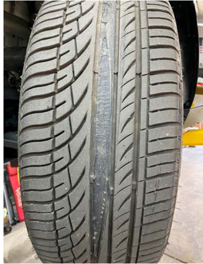
Figure 4 – Major tire damage
