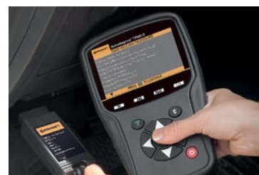
Autodiagnos TPMS D Tool Diagnostics, TPMS service and tire service in one unit.
