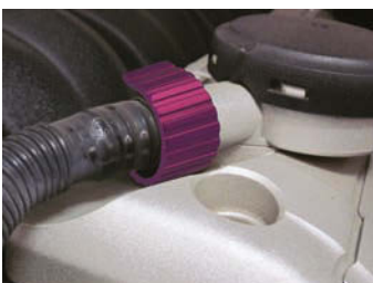
SP Tools/Schley Products Breather Hose Release Tools, No. 14550 CATEGORY: Specialty Tools Enter #72 at "e-inquiry" on VehicleServicePros.com
