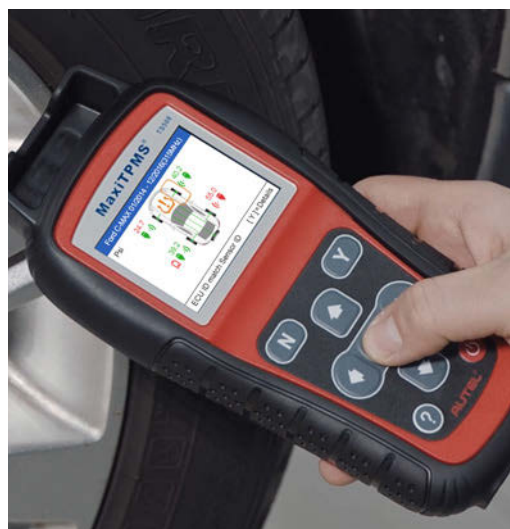
The MaxiTPMS TS508 from Autel features Wi-Fi capabilities for software updates and data transfer. The TS508 can also perform placard adjustments and initiate relearn sequences through the OBD-II port.
