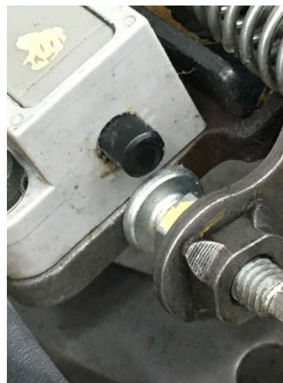
▲ Note in this image the arm is bent, which prevented the brake pedal pressure sensor from sensing changes.
