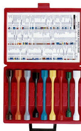
▲ The Ken-Tool Torque Starter Kit, No. 30180, is designed to help technicians easily tighten wheels to the correct torque.
