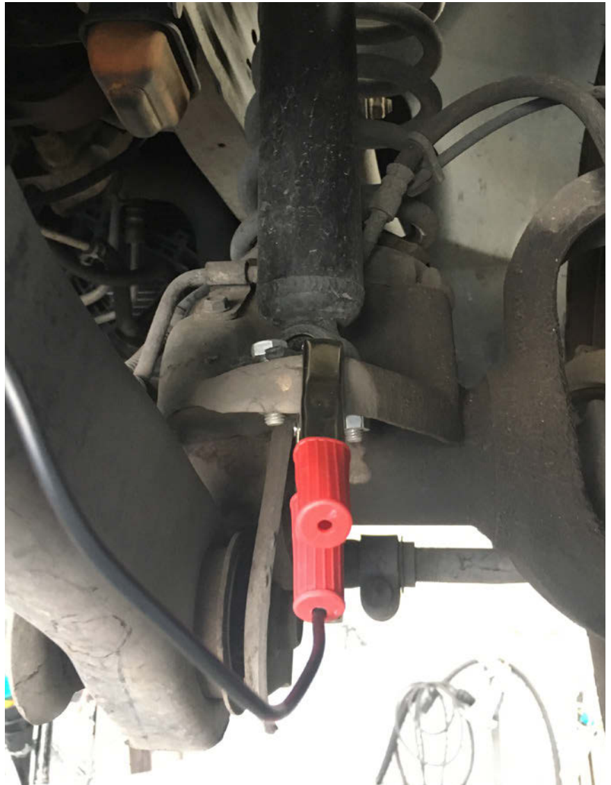
▲ Be sure to place the transmitter and microphone wire in a location away from moving parts and hot exhaust components.
