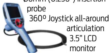
Exchangeable probe camera
