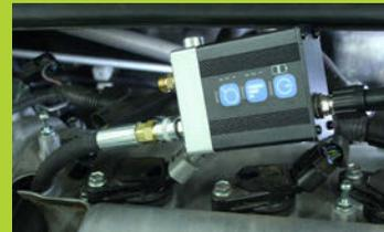
in tested systems, displaying them on a timeline with other related events to make it easier to diagnose vehicle issues and reveals how to repair them. It features an operating range from -15 psi up to 500 psi, and is also auto zeroing, temperature compensated, and noise shielded for maximum set-up simplicity and measurement accuracy.
