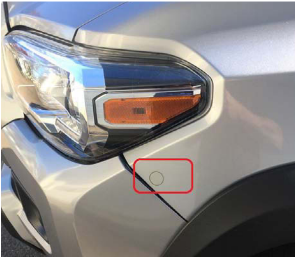
▲ Image of front ADAS sensor on Toyota Tacoma.
