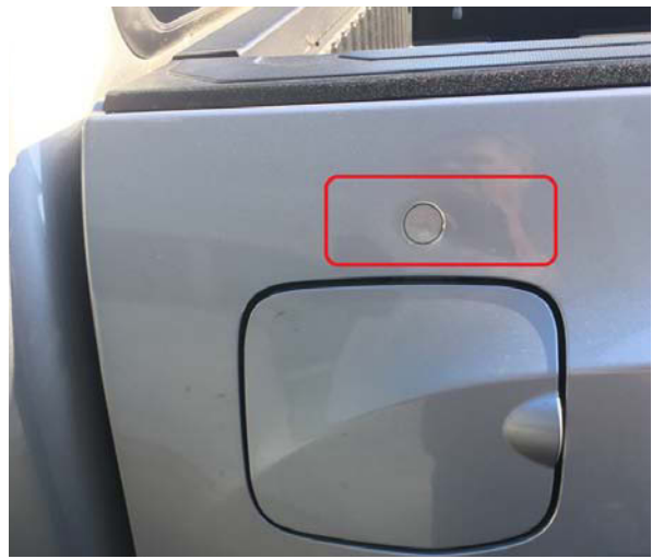
▲ Image of side warning sensor on Toyota Tacoma. It should be noted if paint repairs are done, the original color must be matched.
