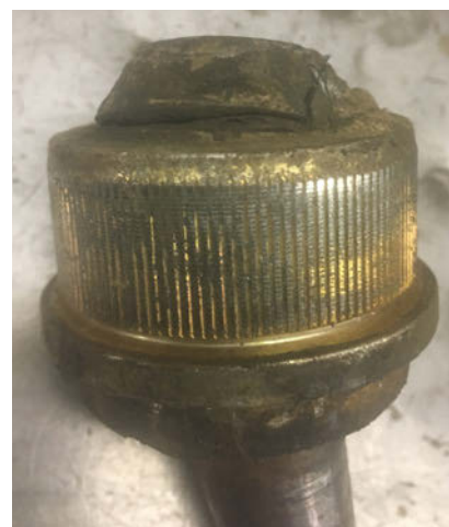
▲ Not every suspension problem is as obvious as this broken ball joint.
