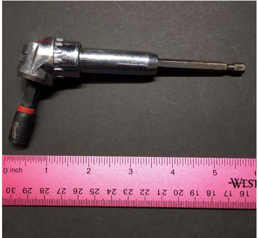
▲ When working under the dash, the Right Angle Screw Bit Adapter from Milwaukee Tools saves valuable time.
