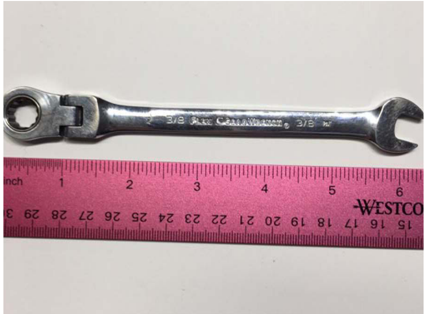
▲ Another time saving and convenient set of tools for working in tight quarters are the Flex Head Wrenches from GEARWRENCH.
