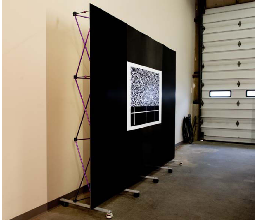
▲ An ADAS target for Subaru, made by OEMTools.com, a division of CAS. Each tool manufacturer will have a minimum and maximum service area size. Shops can check this by placing a vehicle at a prescribed distance from the sensor plates, as laid out by the manufacturer's scanner specifications.
