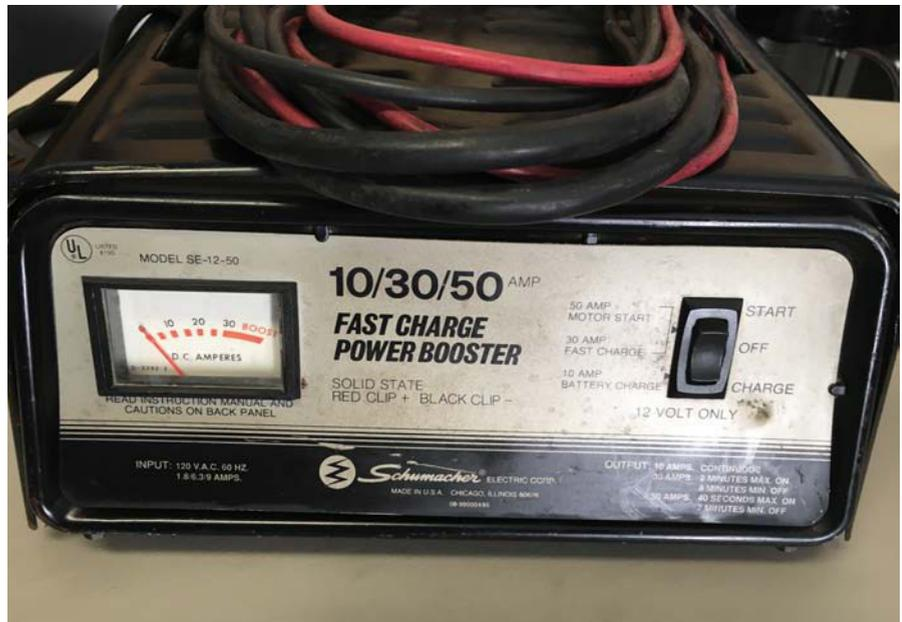
▲ *Small chargers such as this one still have some limited uses, such as slow charging a flooded cell lead acid battery.*
