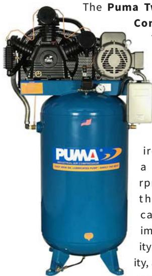
The **Puma Two-Stage Air Compressor**, No. TUK-7580VM, delivers 23 cfm at 175 psi, includes a splash lubricated belt drive, cast iron pump and a 7.5 hp, 1,750 rpm motor. The three-cylinder cast iron pump improves durability and dependability, according to the company. Standard features include a
