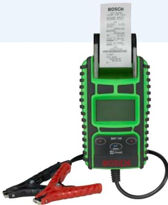
▲ The Bosch BAT 135 battery tester with integrated printer is designed to capture test results for customer records such as presenting the state of health and state of charge percentage of the batteries to ensure optimal efficiency and usage.
