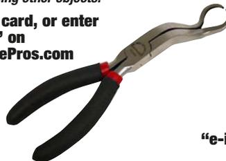
▼ **The Lisle Offset Spark Plug Wire Removal Pliers** can remove the toughest spark plug wires. The 5/8" opening of the pliers properly fits the plug wire boots, preventing damage. The offset design works great on boots with heat sleeves, such as those found on some GM engines. They are easy-to-use in tight places. The pliers can also be used on hoses or for holding other objects.
