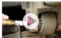
Cleaning clogged grease joints can be troublesome to technicians. IPA Tools demonstrates how the 7863 Grease Joint Rejuvenator Master Kit helps remove old, hardened grease, dirt and debris from clogged bearings. To watch the video demonstration, visit:
