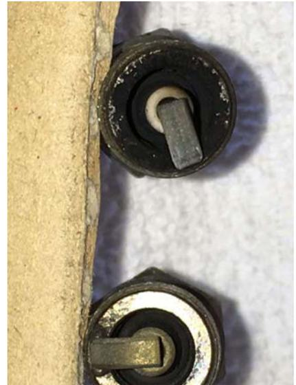
▲ Fig 4. Note the carbon buildup on the spark plug removed from bank 2 is different from the bank 1 plug.
