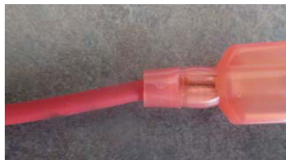
▲ Image of a terminal that has been over-crimped. Notice where the insulator is spread out at the crimp.
