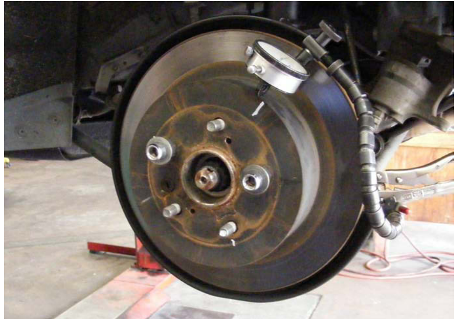
▲ This image illustrates using a dial indicator to check for hub or rotor run out.
