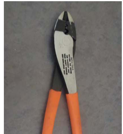
▲ When crimping connectors, make sure to crimp to the correct torque. Crimping too tight will damage the wire, and too loose will create a poor connection. Pictured here is a pair of Matco Tools terminal crimping pliers.
