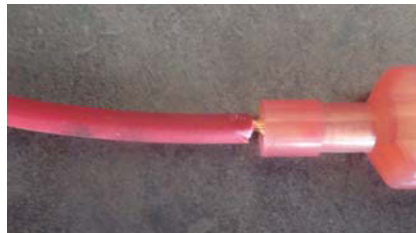
▲ Wire stripped too far will not seat into the crimp housing, and will also leave the wire un-insulated, possibly causing a short.
