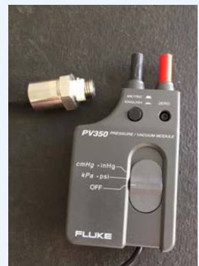
▼ This Fluke pressure transducer is a helpful accessory for use with a lab scope or DMM.
