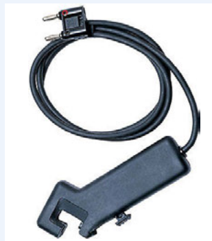
▲ A useful lab scope accessory, inductive pick-up probes for RPM signals are good for quickly analyzing signals that sync to a specific event, such as checking an ignition event compared to the actual crankshaft position.
