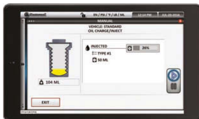
OIL INJECTION SCREEN View real time oil injection and waste oil collection with displayed weights
