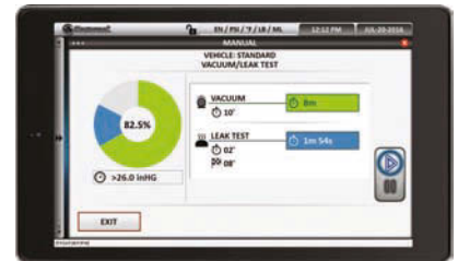
VACUUM SCREEN Fully customizable options allow the user to program vacuum and leak test times
