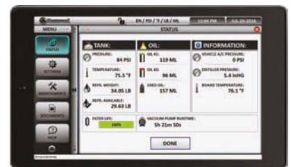
MENU SCREEN/STATUS View all pressures, temperatures, refrigerant and oil weights. View vacuum pump run time and oil change
